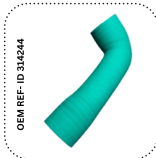
IKO - HUMP - 0104 Eicher L-Bend "2.5"(Double Bend) Hose IC outlet ID "2.5" * "2.5" * "15" Long
